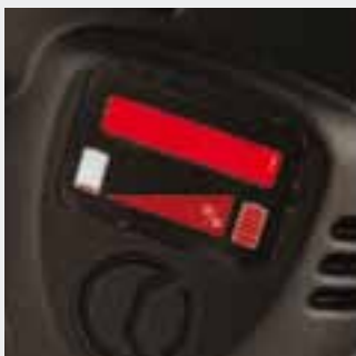
Battery condition display
