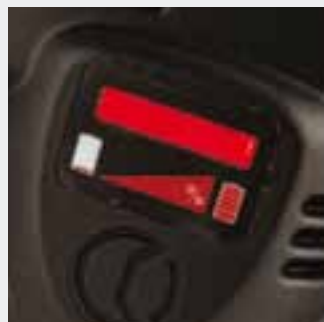
Battery condition display
